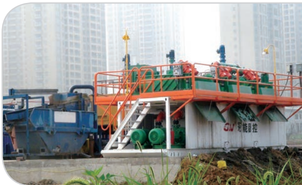
Dredging Slurry Solids and Liquid Separation
