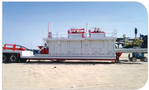
Water Well Drilling Mud Recycling
